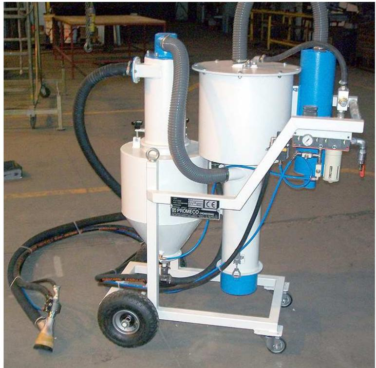
Picture of the sandblasting machine Mod. PR2
